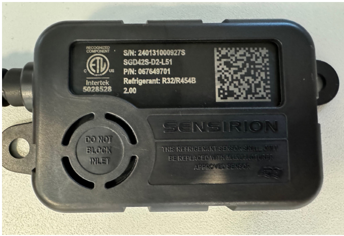
FIGURE 7. Example of Clear, Unobstructed Sensor Inlet
